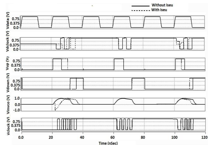
Fig. 13: Simulation Result for complete PLL with and without current pulse ( I_{SEU} ) strike at 22ns.
